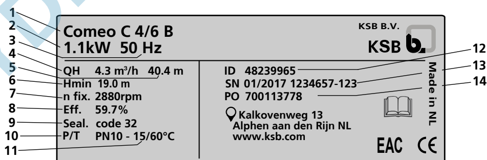
III. 2: Plaque signalétique Comeo (exemple)
