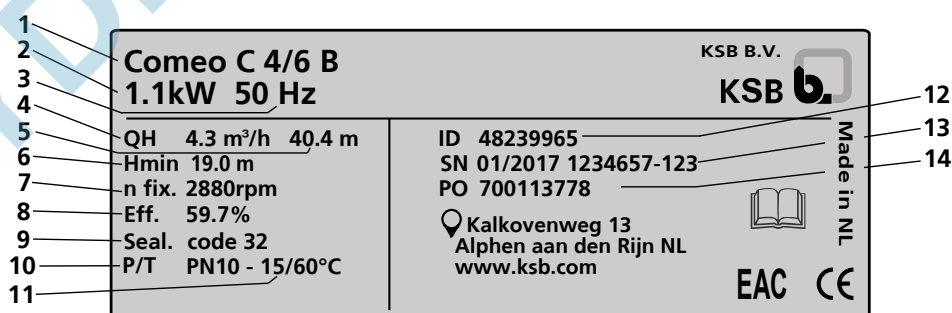
III. 2: Plaque signalétique Comeo (exemple)
