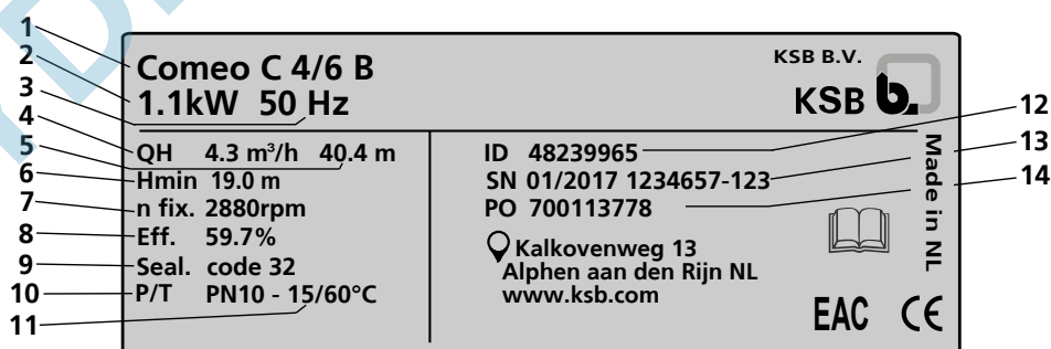
III. 2: Plaque signalétique Comeo (exemple)
